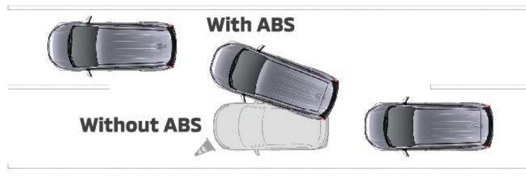
ABS (ANTI-LOCK BRAKING SYSTEM), EBD (ELECTRONIC BRAKE DISTRIBUTION) WITH BRAKE ASSIST (BA)
